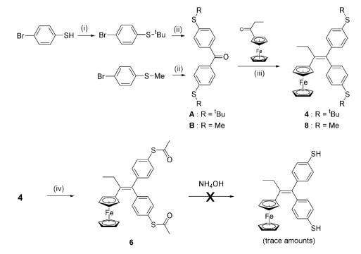
Scheme 1. (i)  $1 - {}^{t}BuCl$ , AlCl<sub>3</sub>, r.t., 1 h and  $2 - H_2O$ ; (ii)  $1 - {}^{n}BuLi$ , Et<sub>2</sub>O  $-30 \circ C \rightarrow -10 \circ C$ , 3 h,  $2 - Me_2NC(O)Cl$ , Et<sub>2</sub>O,  $-50 \circ C \rightarrow 0 \circ C$ , 3 h, and  $3 - NH_4Cl$ , H<sub>2</sub>O; (iii)  $1 - TiCl_4/Zn$ , THF, reflux, 3–6 h and 2 – HCl, H<sub>2</sub>O; and (iv) 1 – exc. BBr<sub>3</sub>, exc. H<sub>3</sub>CC(O)Cl, CH<sub>2</sub>Cl<sub>2</sub>, r.t., 6 days and 2 – NaHCO<sub>3(aq)</sub>.
