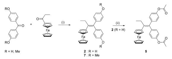
Scheme 2. (i) 1 - TiCl<sub>4</sub>/Zn, THF, reflux, 3 h and 2 - HCl, H<sub>2</sub>O and (ii) 1 - exc. H<sub>3</sub>CC(O)Cl, CH<sub>2</sub>Cl<sub>2</sub>, r.t., 12 h and 2 - H<sub>2</sub>O.
